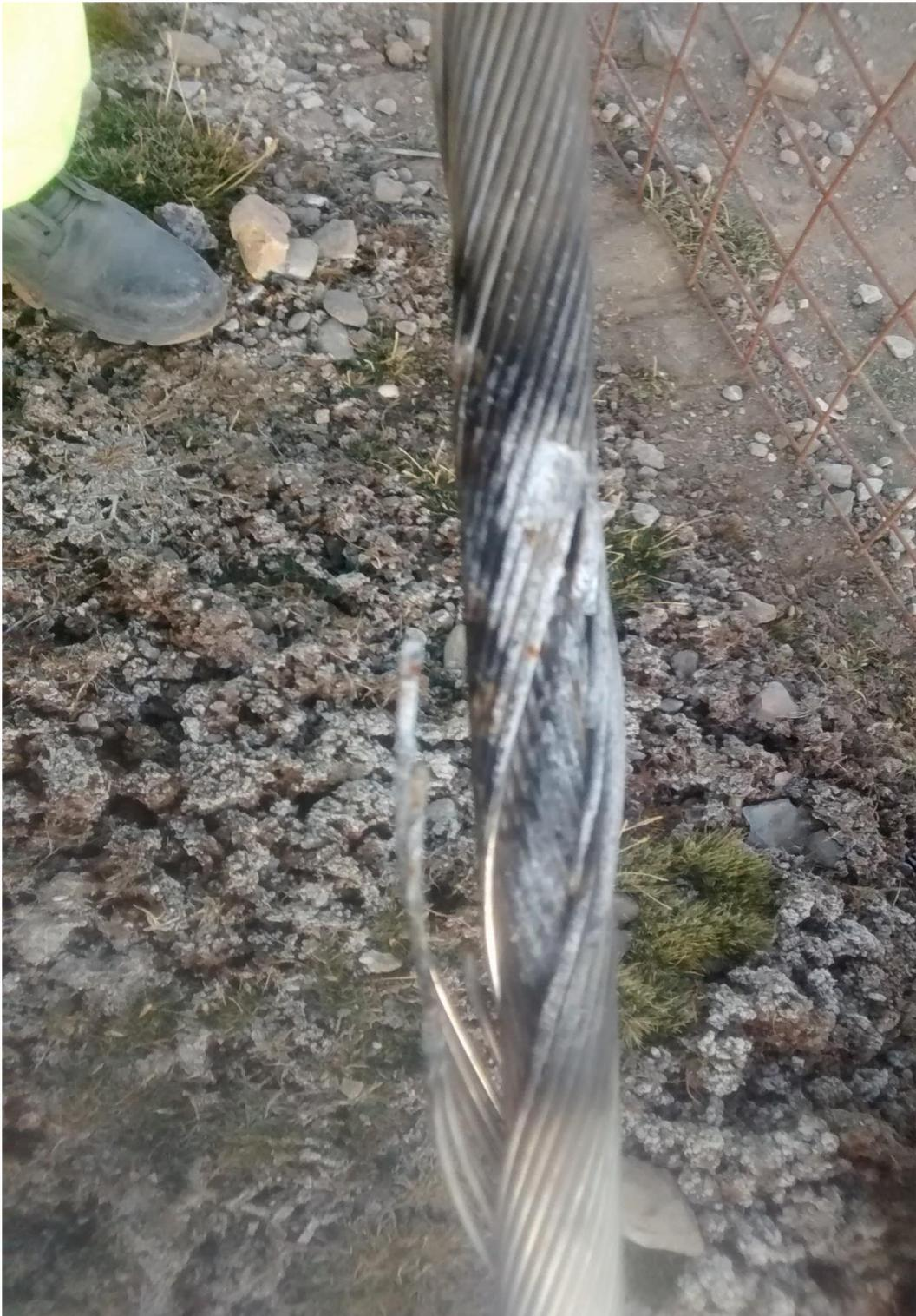
**FIG.32 TRAMO DEL CONDUCTOR DAÑADO POR LA DESCARGA ATMOSFERICA DIRECTA
